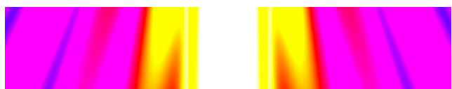
Cross-section of the modelled i-line (365 nm) exposure intensity distribution in a 2 µm thick resist film and a 2 µm slit in the photomask with no (top) and 10 µm (bottom) proximity gap.
