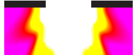
Cross-section of the modelled i-line (365 nm) exposure intensity distribution in a 1 µm thick resist film and a 1 µm slit in the photomask.
