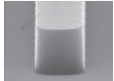
1 µm AZ<sup>®</sup> 701 MiR line after 130°C hardbake
