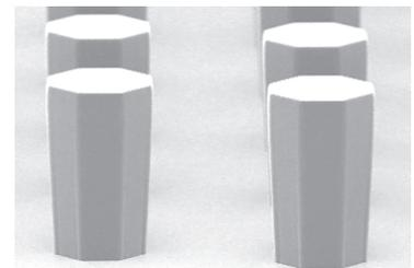
120 µm plated Cu-coloums (with the AZ<sup>®</sup> 125 nXT)
