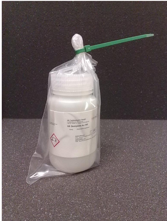
Closing the bag with a zip tie forming a loop with the open end
