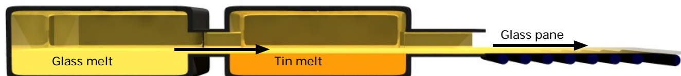
Fig. 37: The production of glass panes in the "float process" technique
