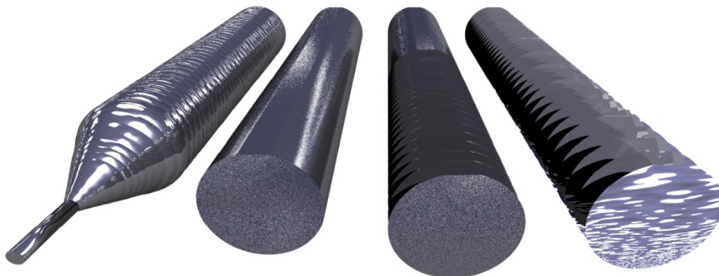
Fig. 15: Grinding, sawing, etching and polished (from left to right) are the work steps from an ingot to a finished wafer
