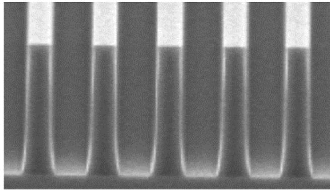
2.4 $\mu\text{m}$  lines in 10 $\mu\text{m}$  thick AZ 12XT
