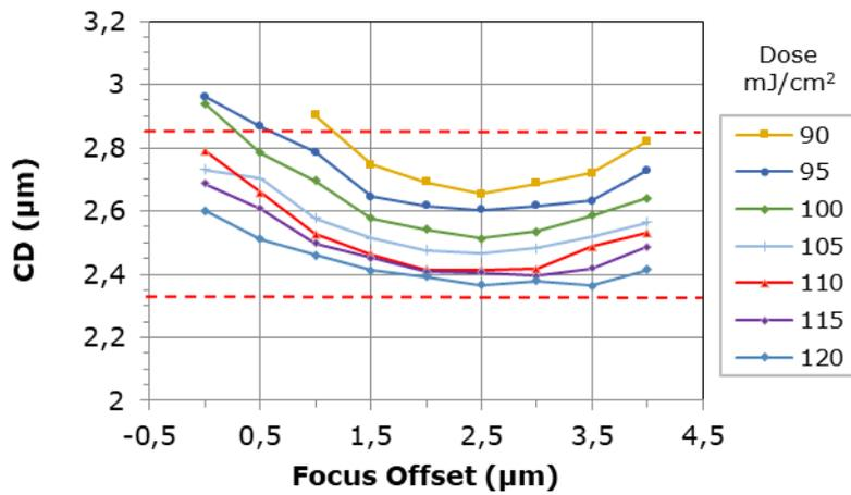
Mask CD: 2.6µm lines @ 1:1 pitch
