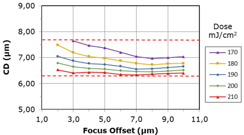
Mask CD: 7.0µm lines @ 1:1 pitch
