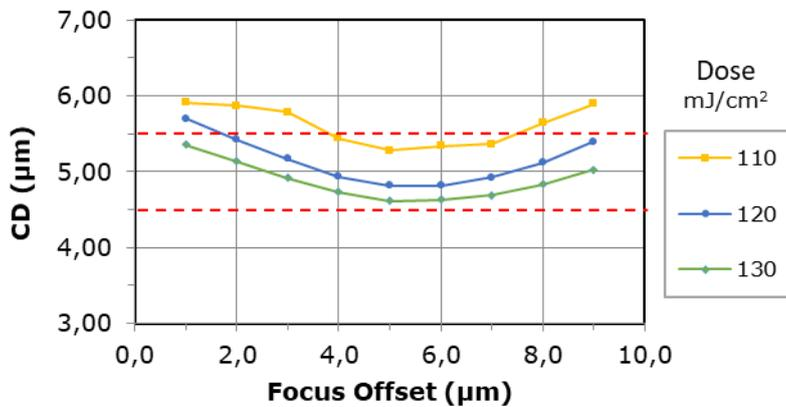
Mask CD: 5.0µm lines @ 1:1 pitch
