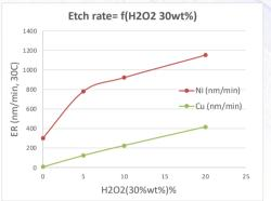
Etch rate (nm/min) for Cu and Ni blankets = f( Temperature and H2O2 content)
