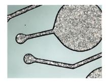
UBM (AU/Cu/Ni) and RDL (Cu seed/Cu) applications
