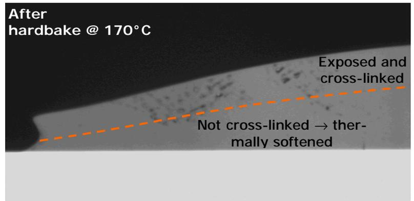
One way to stabilize even thick films of AZ<sup>®</sup> nLOF is an extended 1<sup>st</sup> exposure. However, this will reduce the lateral resolution and require unreasonable high exposure times in case of films exceeding 10-15 µm.
