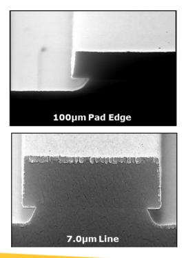
AZ ECI 3012 Photoresist Post Oxide Etch Resist Thickness: 1.33µm Primer: HMDS vapor Soft Bake: 90°C, 60s contact hot plate Exposure: Suss MA 56 Aligner Post Expose Bake: 110°C, 60s contact hot plate Develop: AZ 300MIF, 60s single puddle
