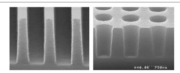
AZ ECI 3012 Photoresist 0.4µm lines and 0.5µm holes 1.20µm thick film 0.54NA i-line exposure AZ 300 MIF Develop (60S)
