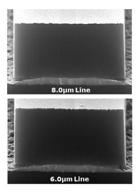
AZ ECI 3012 Photoresist Post ITO Etch Resist Thickness: 1.7μm Soft Bake: 90°C, 90s proximity hot plate Exposure: Nikon Stepper, 0.54NA Post Expose Bake: 110°C, 90s proximity hot plate Develop: AZ 300MIF, 60s single puddle
