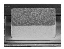
96µm gold bump plated in AZ P4620 Cyanide electro-plating solution
