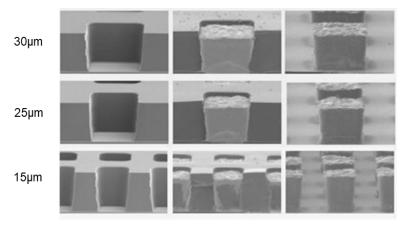
Resist: AZ P4620 Thickness: 24µm Develop: AZ 400K 1:3 Plating Temp: 45C Plating Time: 50 min. Metal Thickness: 20µm
