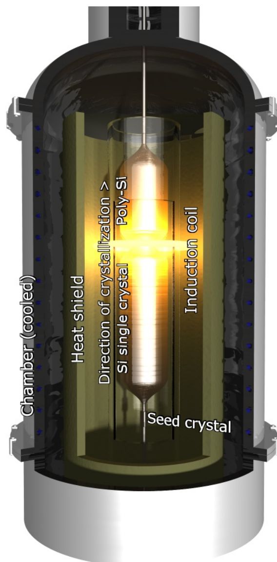
Fig. 5: In zone melting techniques ( Float zone ), an induction coil melts a poly-crystalline silicon crystal longitudinally, which subsequently solidifies in a mono-crystalline manner.
