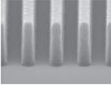
300 nm lines and spaces with the AZ® 701 MiR @ 0.8 µm
