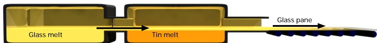
Fig. 37: The production of glass panes in the "float process" technique
