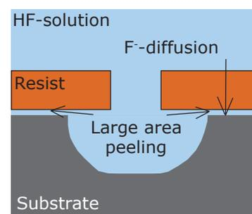
F<sup>-</sup>-ions diffuse through the resist film towards the substrate, etch the substrate material, followed by a large-scale resist peeling.
