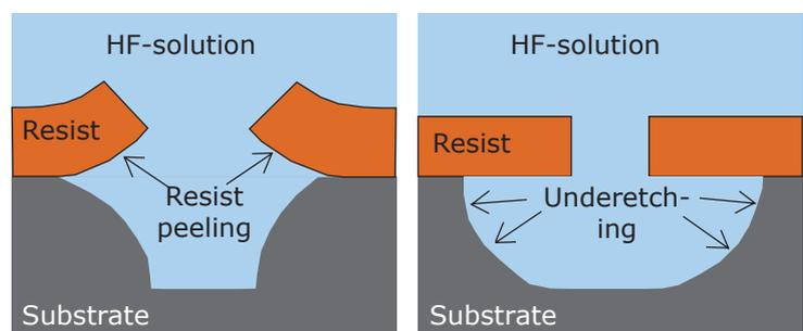
The etched profile reveals if either the resist adhesion is poor (left), or only the inevitable underetching in case of isotropical etching occurs (right).
